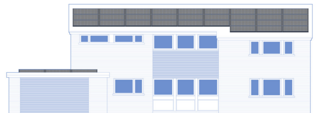
Example of a solar panel array on the front elevation as well as an array on the flat-roofed garage
