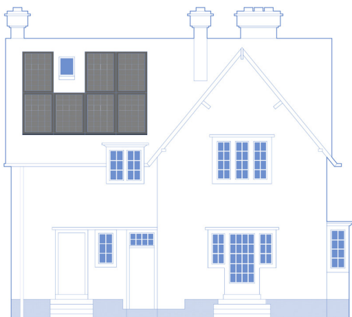
An example of an orderly solar panel array arranged around an existing rooflight. Note that the overall shape of the array remains rectangular.
