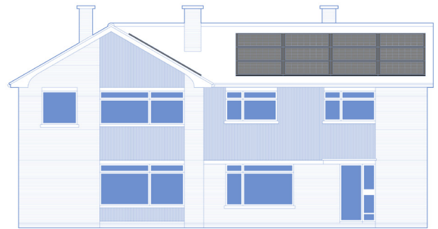
An example of a balanced, rectangular solar panel array positioned on the front elevation.
