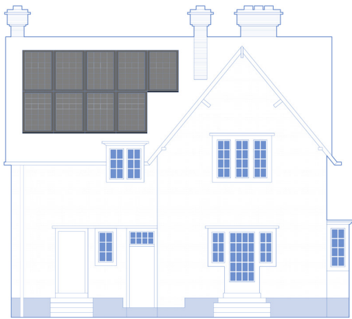
An example of an orderly solar panel array arranged in a staggered formation to follow the form of the roof.
