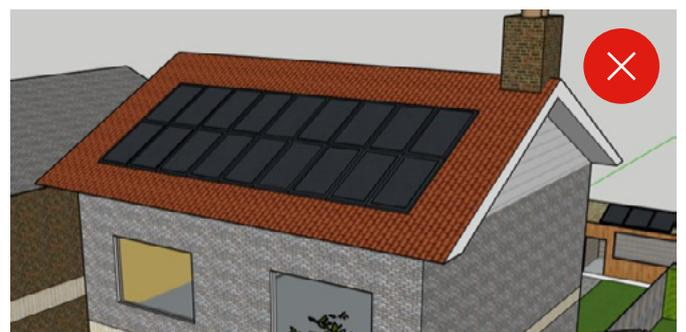
This (above) installation is also unacceptable in the HCA. Though the array is proportioned and rectangular, it is located on the street-facing roof pitch.
