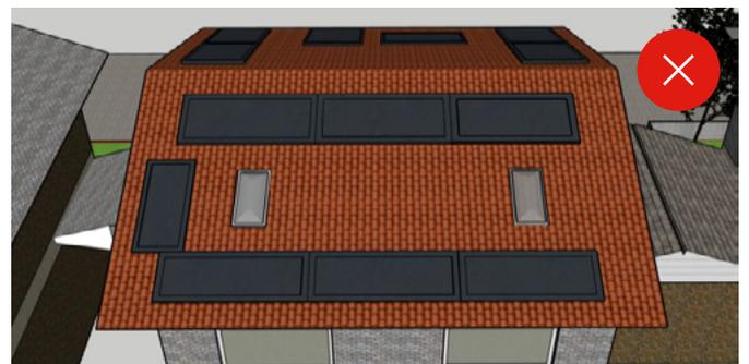
The Foundation discourages L-shaped installations such as the example above.
