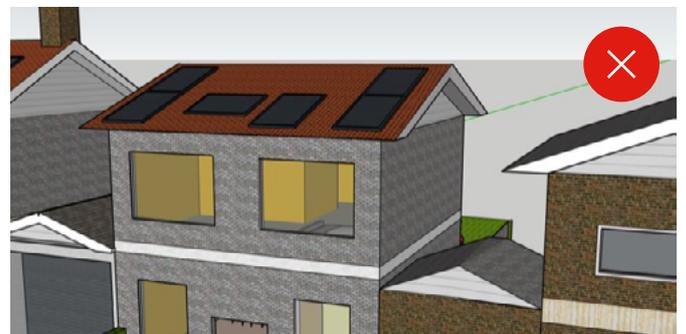
This array would not be acceptable in the MCA. Although installation is permitted on the front, street-facing roof pitch, the design itself is poor. The panels are disconnected, facing different directions, and unbalanced.
