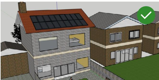
The above represents good installation in the HCA. It is located on the rear roof pitch with a balanced, rectangular design.
