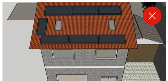
The Foundation discourages L-shaped installations such as the example above.
