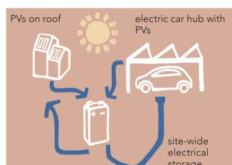
The site-wide energy strategy is based around on-site energy generation and storage. Photovoltaic tiles (PVs) on southfacing roofs of the houses generate electricity, which is used by households and stored during periods of low demand in batteries distributed throughout the green corridors. The solar roof of the car hubs generates electricity to charge electric cars at a reduced rate for residents, creating additional incentive to park in the hubs.
