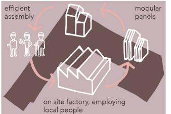
within the community, and reducing transportation during construction. CLT modular timber construction will be used to lower the carbon ootprint, reduce construction time and create less wastage. This type of construction also lends itself well to self build. The factory building will be re-purposed as a community facility, such as a sports hall.
