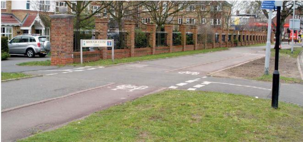
Figure 5.17: Example of cycle track priority over junction mouth
