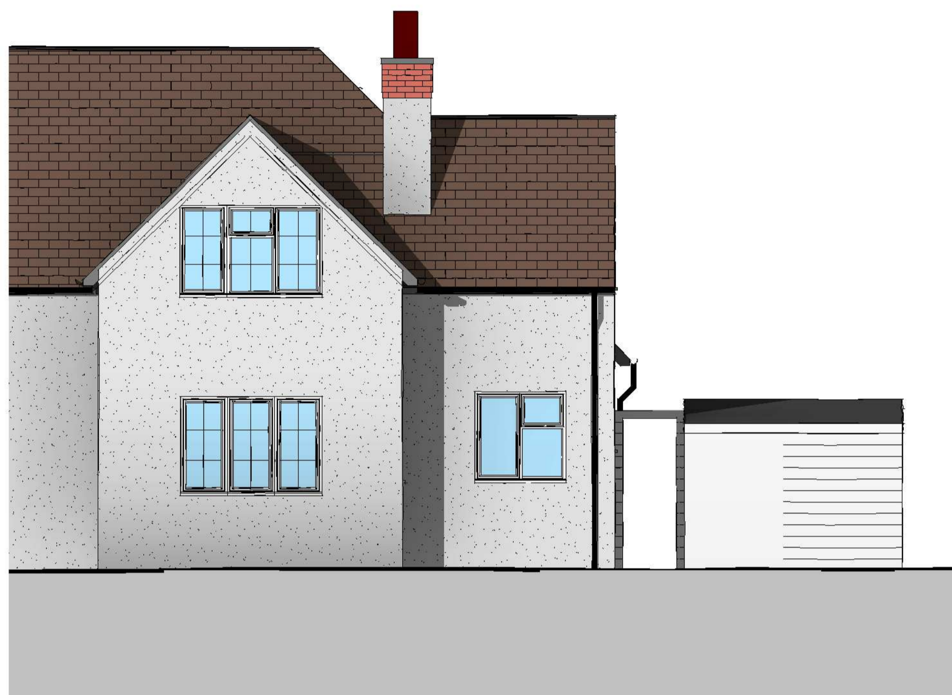
Rear Elevation - Existing 1 : 50
