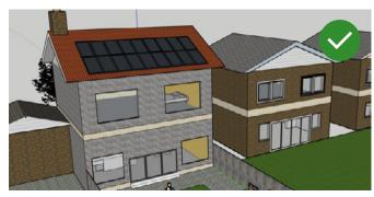
The above represents good installation in the HCA. It is located on the rear roof pitch with a balanced, rectangular design.
