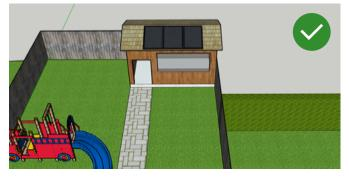
Installations placed on outbuildings, like this, represent viable alternatives to an unsuitable rear roof pitch in the HCA. As with main roof arrays, balanced design is key.
