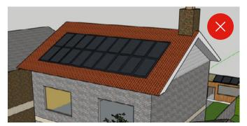
This (above) installation is also unacceptable in the HCA. Though the array is proportioned and rectangular, it is located on the street-facing roof pitch.
