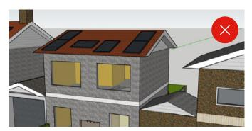
This array would not be acceptable in the MCA. Although installation is permitted on the front, street-facing roof pitch, the design itself is poor. The panels are disconnected, facing different directions, and unbalanced.
