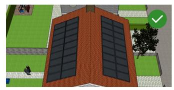
Providing that the installation is balanced (rectangular or straight-lined), it is permissible to introduce PV panels to both the rear and street-facing roof pitches (see above).
