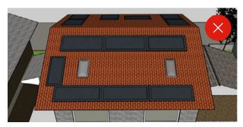
The Foundation discourages L-shaped installations such as the example above.
