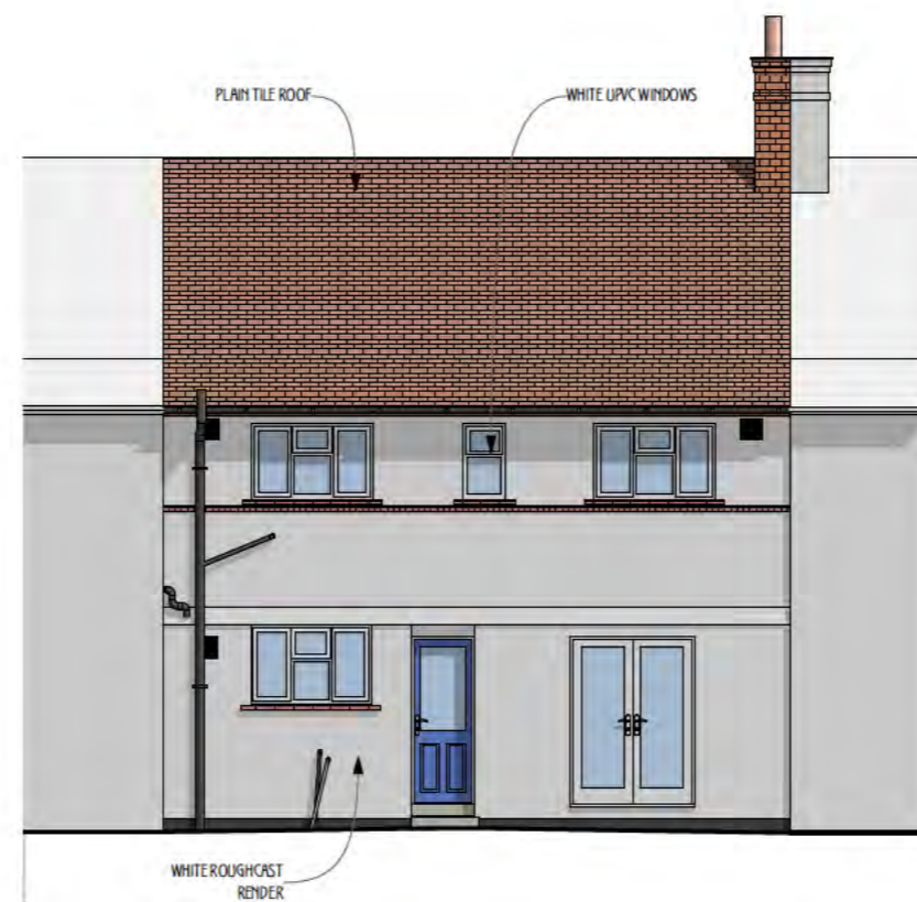
E-02 North West Elevation 1:100
